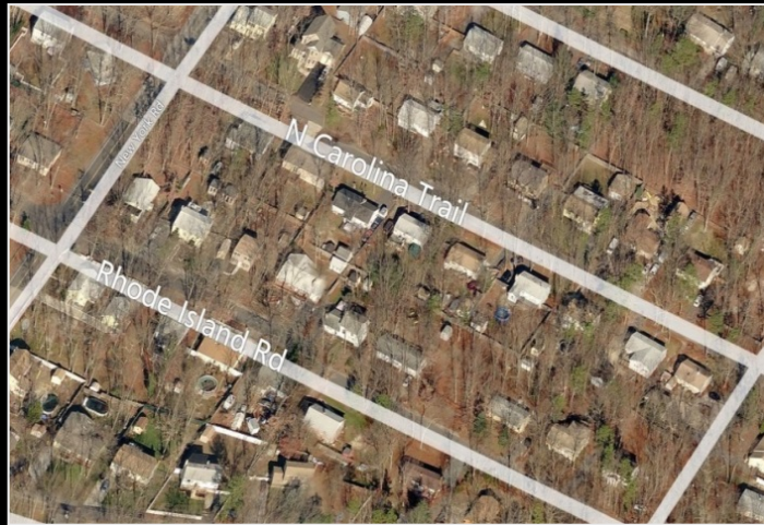
High density residential development on septic systems & wells (potable water well contamination threat)
